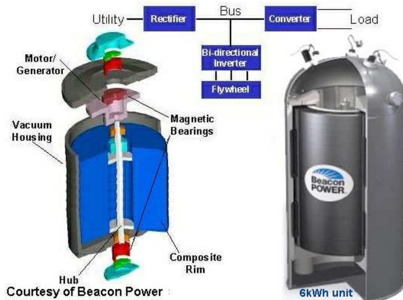
Figure 2.14. Flywheel Cross-Section [44]
